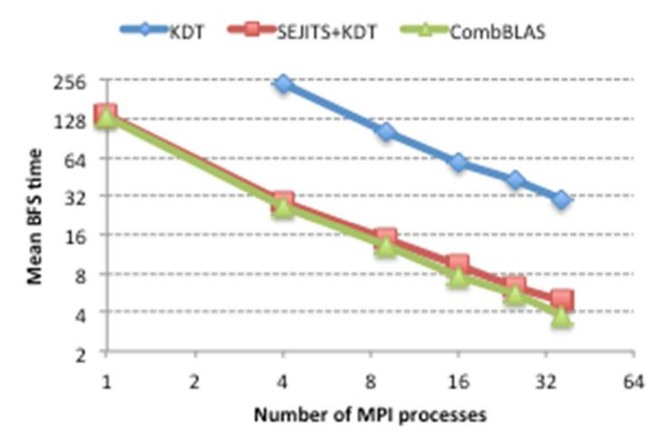
Time (in seconds) for a single BFS iteration on Scale 23 RMAT (8M vertices, 130M edges) with 10% of elements passing filter. Machine is Mirasol.
